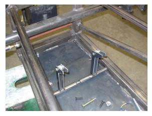
**Status Report:** Our car is coming along quite nicely. At this point we have the gas and brake pedals created and are mounted in the car. We have also finished out kill switch plate and have a mount for the starter button. Zak was able to get a racing seat from his uncle that we have been able to modify to make it easier to get in and out of the car.
